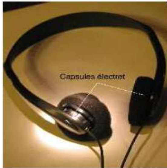
Fig. 14 The “phonocasque” used for the binaural recordings
