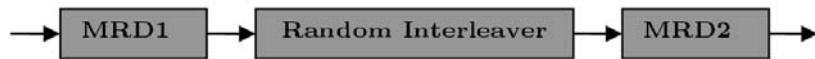
Figure 12. Block diagram used at the source node to encode. The horizontal direction is encoded twice allowing to have more redundancy symbols and, therefore, larger correction capacity.
