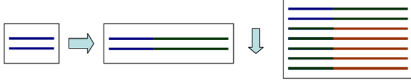
Figure 6. Schematic encoding procedure for product codes. The encoding in vertical and horizontal directions is depicted.
