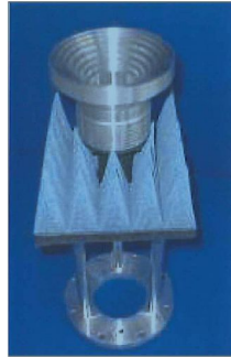
Figure 3.2.: Example of corrugated horn used as CR feed. Taken from ORBIT/FR datasheet [17].
