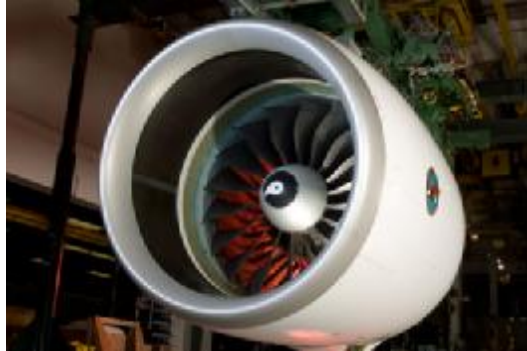
Fig. 10: Pratt & Whitney's Geared Turbofan demonstrator engine during a nacelle system fit check. [5]
