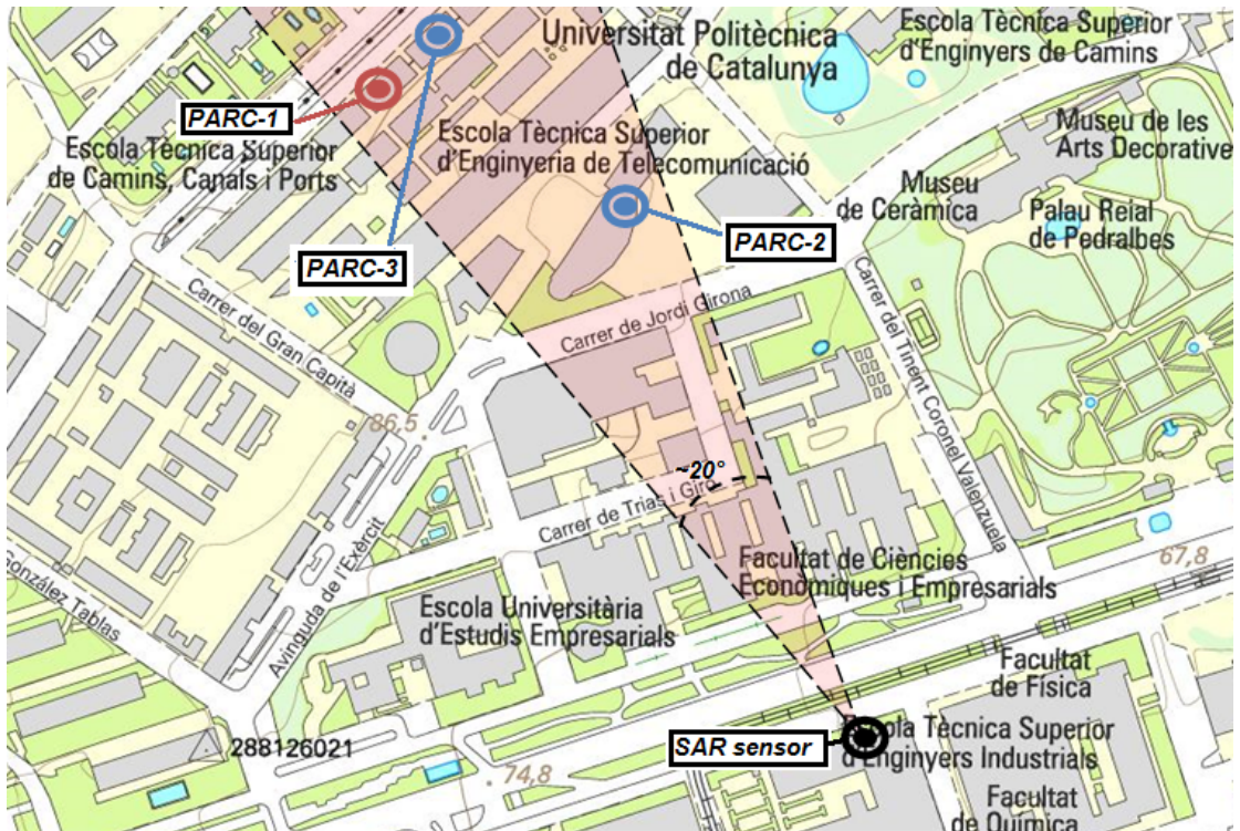
Figure 4.9: Location of the three PARCs and SAR detector. Red dot denotes the ONE-PARC configuration, and Blue dots denote the Two-PARC configuration. The shadowed area represents the 20^\circ beamwidth of the SAR sensor's antenna.
