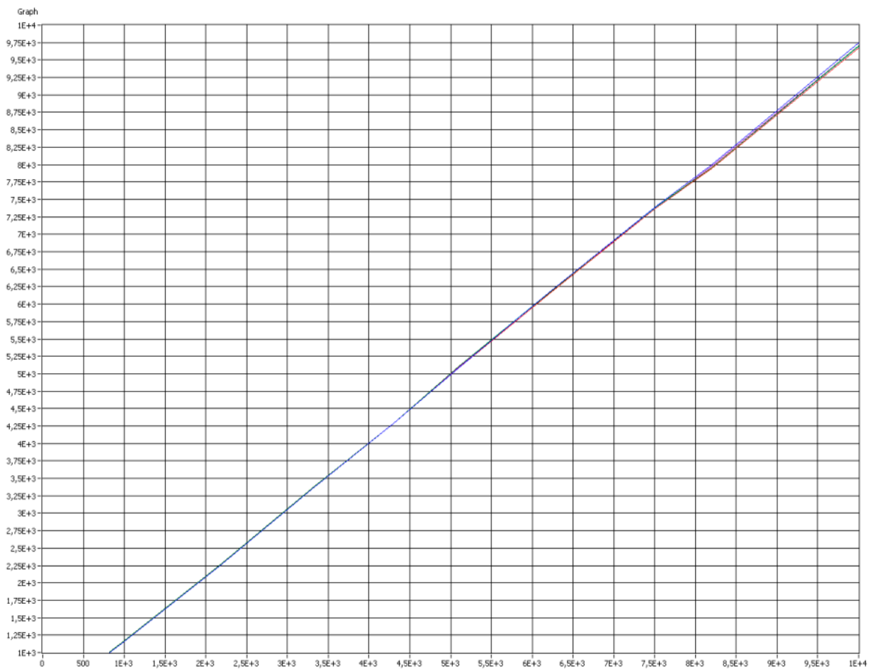
Fig.4.3. Theoretical Resistance vs. Measured Resistance for several frequencies: 5kHz, 25kHz, 50kHz, 75kHz and 100kHz. As observed, a frequency-dependence does not exist except of high values.
