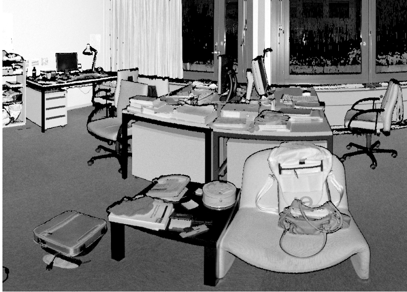
Figure 2.6: The reflection map. The points with no reflection are shown as black points.
