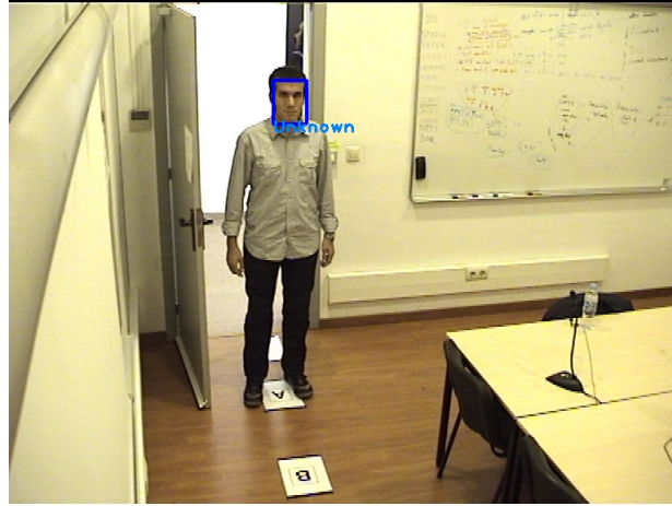
Figure 7.2: Example frame of a training sequence where faces and their identities are still unknown. After detecting the face, a bounding box is created and draw_face_info draws a rectangle around it.
