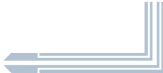
Fig. 2.3 Scheme of a pitot tube.
