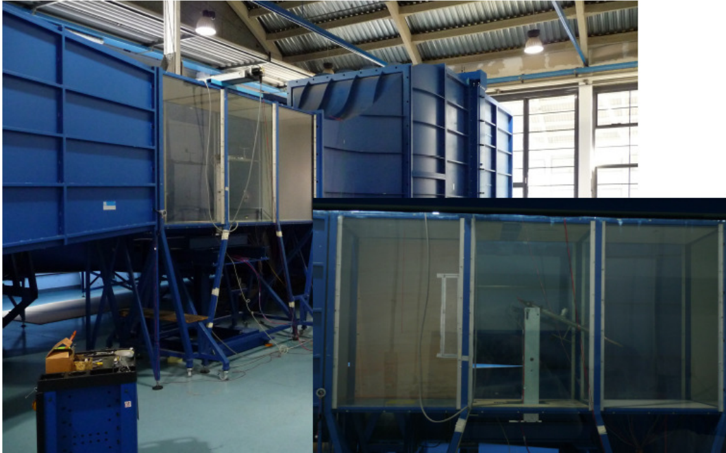
Fig. 5.21 General picture of the wind tunnel and detail of the probe chamber with the boom installed.
