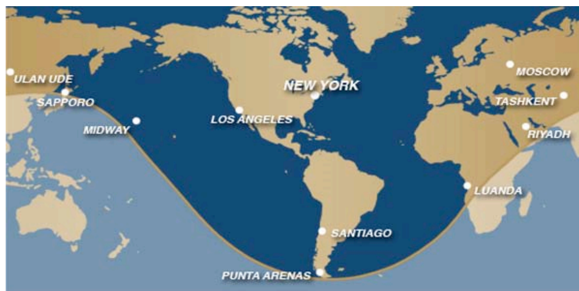
FALCON 7X RANGE FROM NEW YORK 8 passengers, 85% wind reliability, NBAA IFR Reserves
