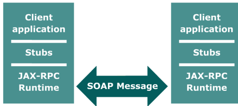
Figure 4.9: illustrates how JAX-WS technology manages communication between a Web service and client.
