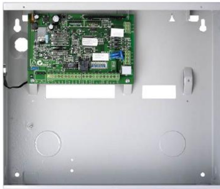
Fig 2.1 Bosch Alarm Central
