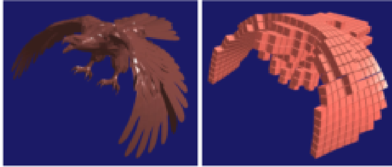
Figure 6.9: Hexahedral finite element volumetric representation of a topologically inconsistent mesh, ready for FEM application (notice that each hexahedron is one of the E_j subdivisions or elements); source [phy5].
