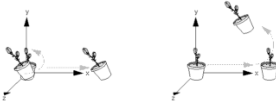
Figure 9.5: The order of the multiplying applied geometric transformations is important: it's not the same a translation applied to a rotation (left) that a rotation applied to a rotation (right); source [gpuE].
