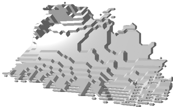
(c) The ForceReaQTor's autogenerated triangular mesh from the mass-spring system volume with Marching Cubes.
