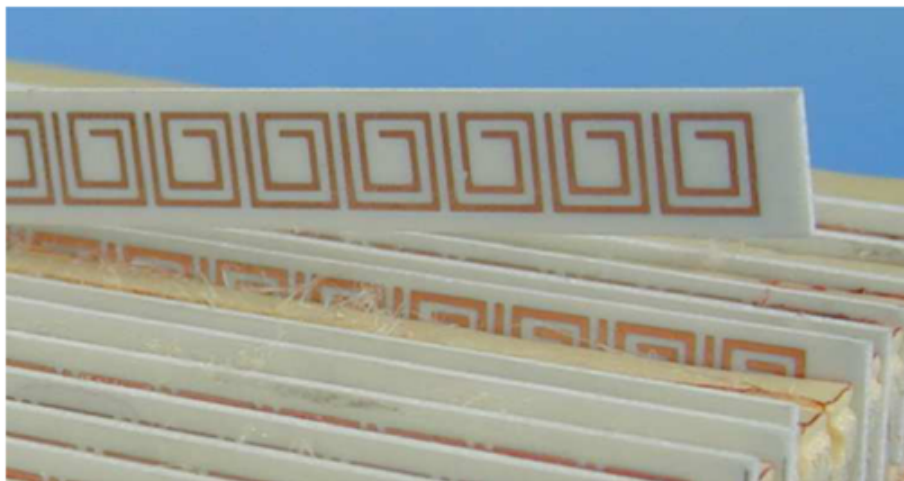
Figure 4.2: Fabricated single layer SR on a Styrofoam board. Fig. from [35].
