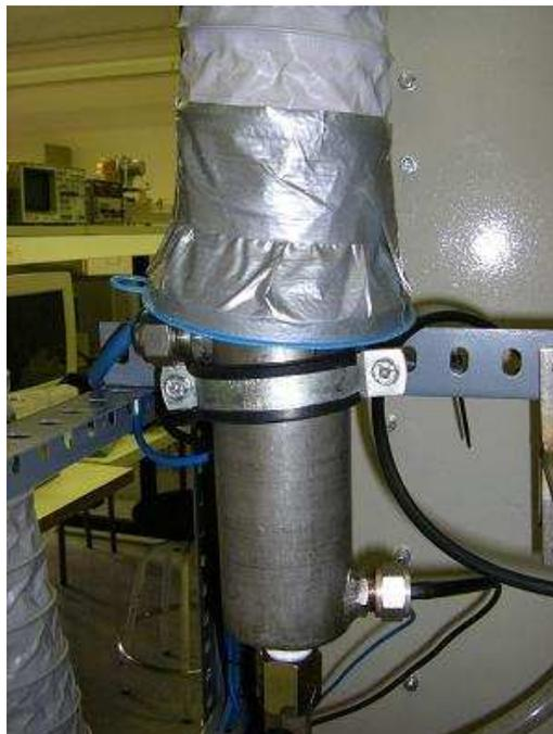
**Figura 30** Extractor de gases
