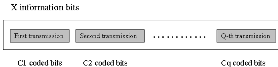
Figure 32 Example of a codeword where no bits will be sent more than once
