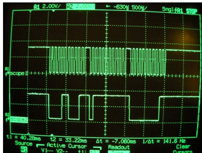
Figure 42. 3 bytes sent from the mouse when movement to the right has occurred
