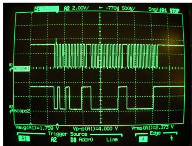
Figure 30. Three bytes sent from the mouse when Left Button is pressed
