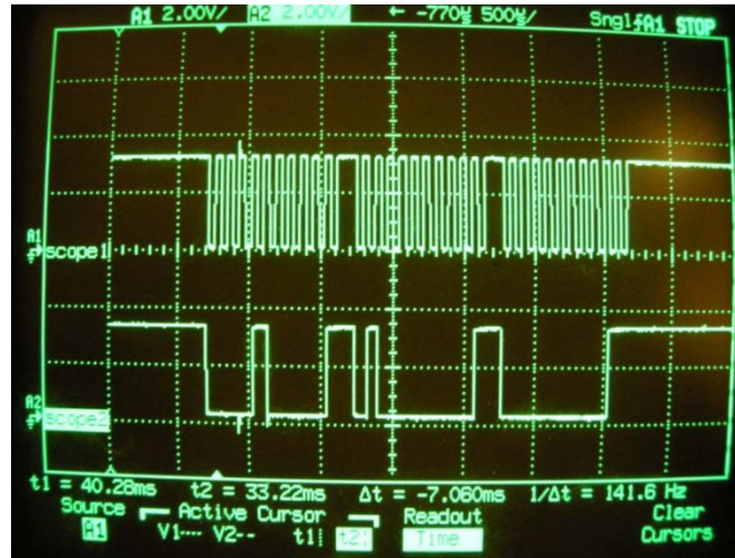
Figure 38. 3 bytes sent from the mouse when moved towards the X direction
