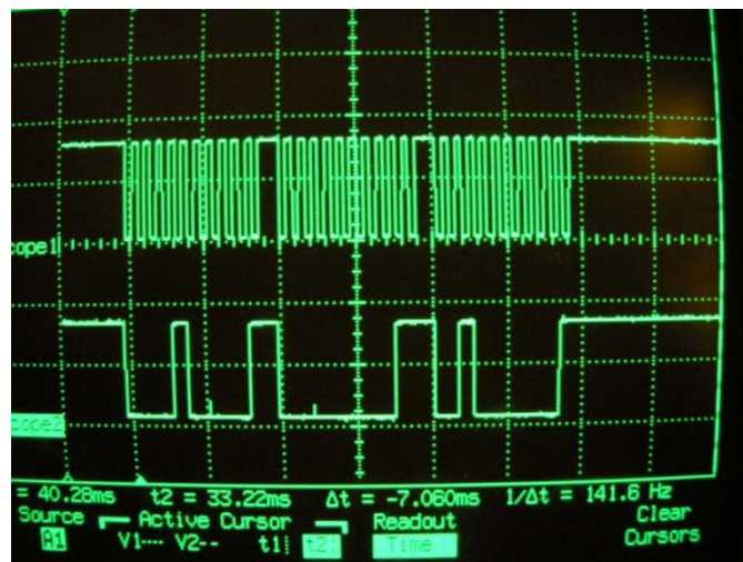
Figure 46. Up movement. 3 bytes sent from the mouse
