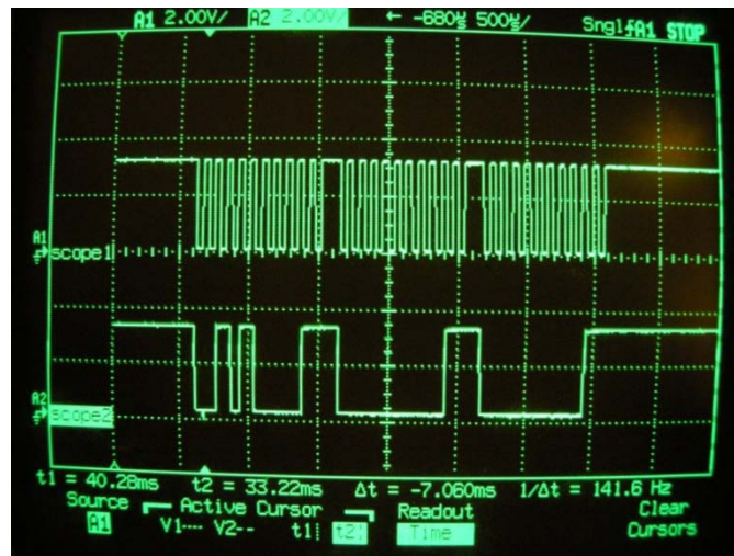
Figure 34. Three bytes sent from the mouse when right button is pressed
