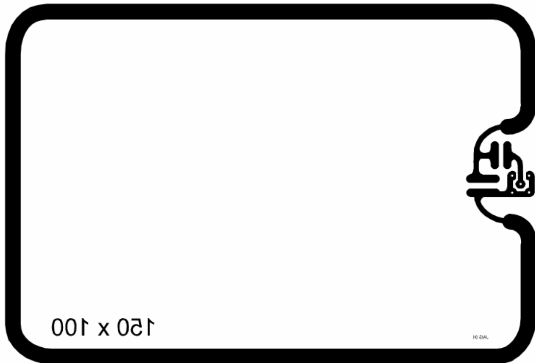
Fig. A1.1 Layout of the custom RFID antenna
