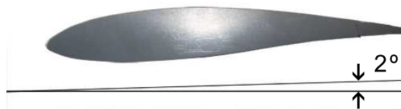
Figure 6.2: Angle on the outer side of the wing of the UAV Shadow
