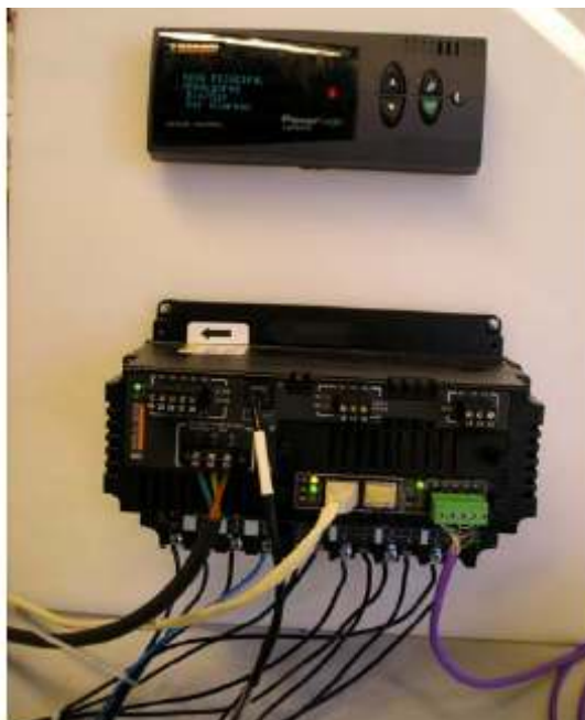
Figure 5.7. CM4000 with card ECC21 and display
