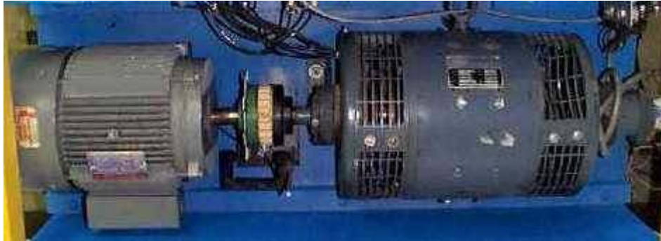
Figure 4.3. 5 HP, 3-phase motor on the left, coupling, DC Generator on the right
