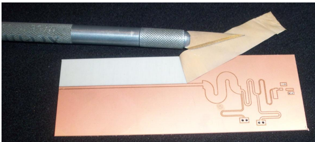
Fig. 4.7.1: Recent fabricated matching-rectifier circuit with copper excess.
