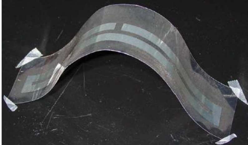
Fig. 5.1.3: Flexible folded dipole made from electro-less silver deposited on a PET substrate [24]
