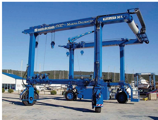
Figure 9.4 : a travel lift for parking nacelle
