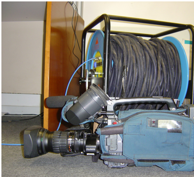
Figure 3.33: Composite video from camera going through 150m of RG-11 cable
