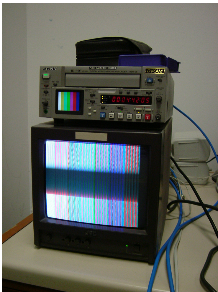
Figure 3.32: Video signal after 300m of VK-7 coaxial cable
