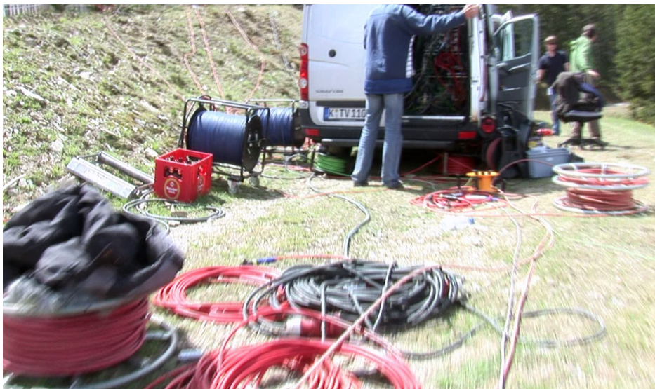
Figure 3.19: Eurosport's OB van with triax cable rollers
