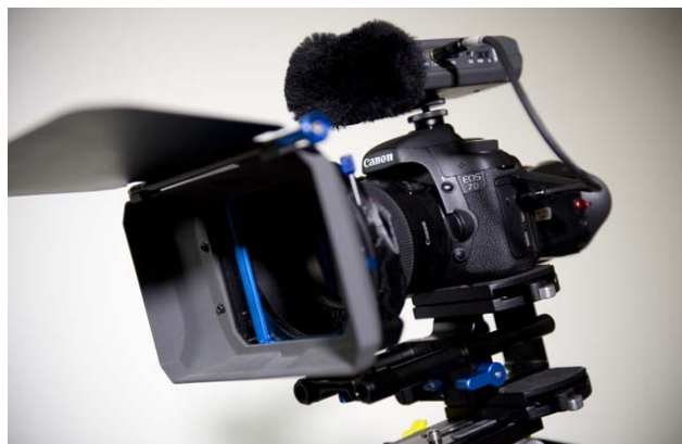
Figure 3.12: Canon EOS 7D APS-C sized HD SLR with a matte box kit
