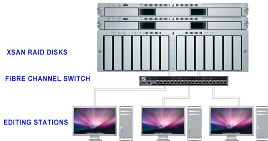
Figure 7.1: Apple Final Cut Server collaborative editing system with XSAN raid disk storage
