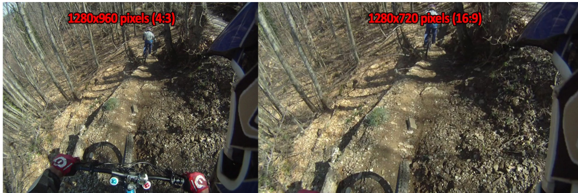
Figure 3.7: Comparison of the angle of view of the 960p and 720p modes
