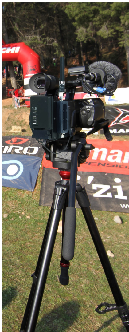
Figure 3.34: Camera with wireless video transmitter
