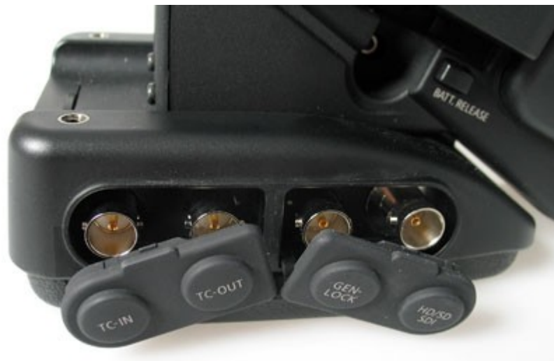
Figure 4.15: BNC timecode input and output from a broadcast camcorder
