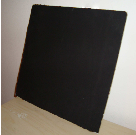
Figure 6.4: Photograph of the 30x30 cm detector screen obtained by coating a piece of poster board. A resistance of 250 \Omega was obtained.
