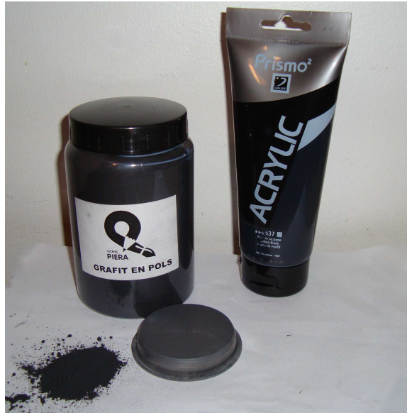
Figure 6.1: Graphite powder and acrylic paint were combined to create a resistive paint.
