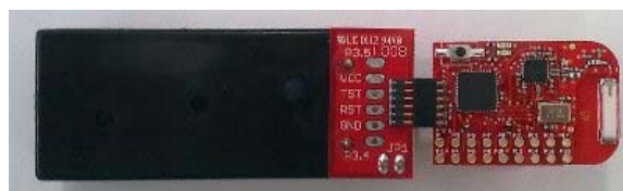
Fig. 4.10 eZ430_RF2500 in a stand-alone system
