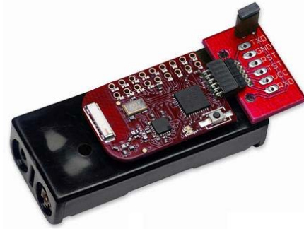
Fig. 4.12 eZ430_RF2500 in a stand-alone system
