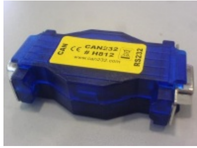
Fig. 2.4 CAN to RS232 converter for PC computer
