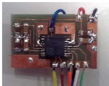
Fig. 5.9 Board with SCA3000-E05 accelerometer
