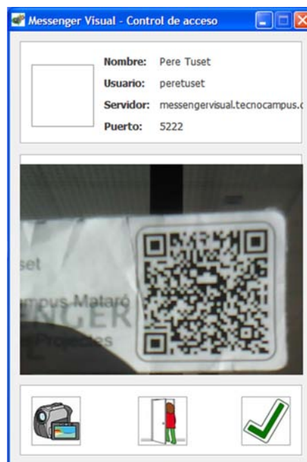
Figure 5.2: The access control mechanism based on QR Codes. The access control window contains a frame that displays the video feed from the camera. A background thread captures still images from the video feed and tries to find and decode a valid QR Code. Once the QR Code is decoded it triggers the login mechanism to authenticate the user to the IM service.
