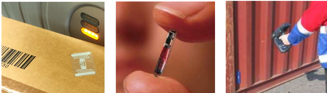
Image 4. Examples of different elements of the RFID Technologies (a-passive Tag; b-active Tag; c-RFID reader)
