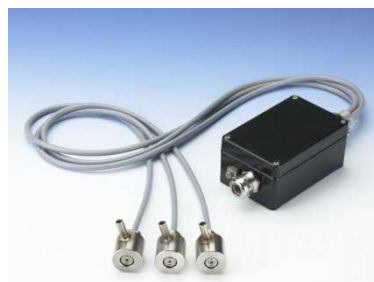
Image 3. Sensor to detect flammable chemical elements
