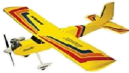
Figure 2.1: Megastar XL120 a giant RC model converted in UAV by Icarus team.
