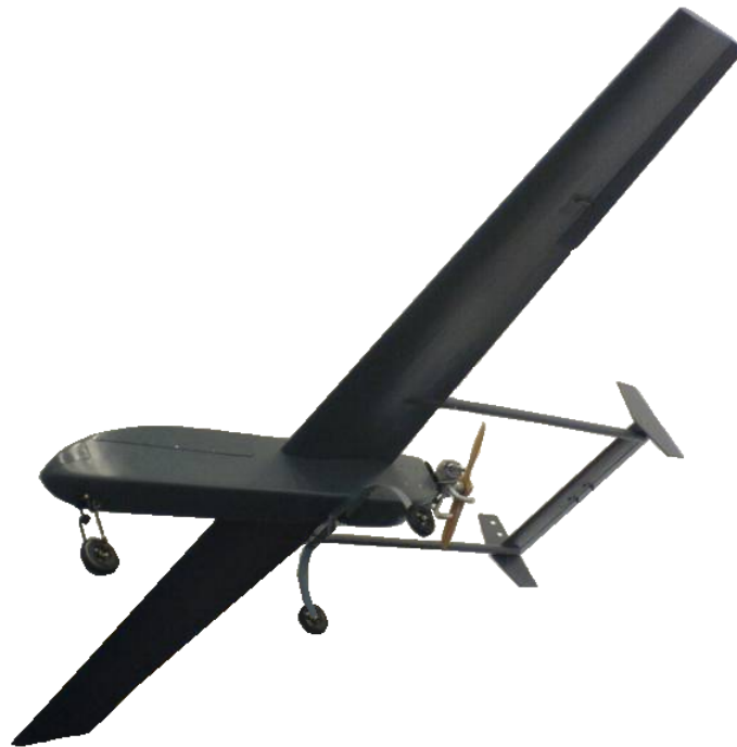
Figure 2.2: Shadow UAV is 17 feet (5.2 meters) of wingspan by Icarus team.
