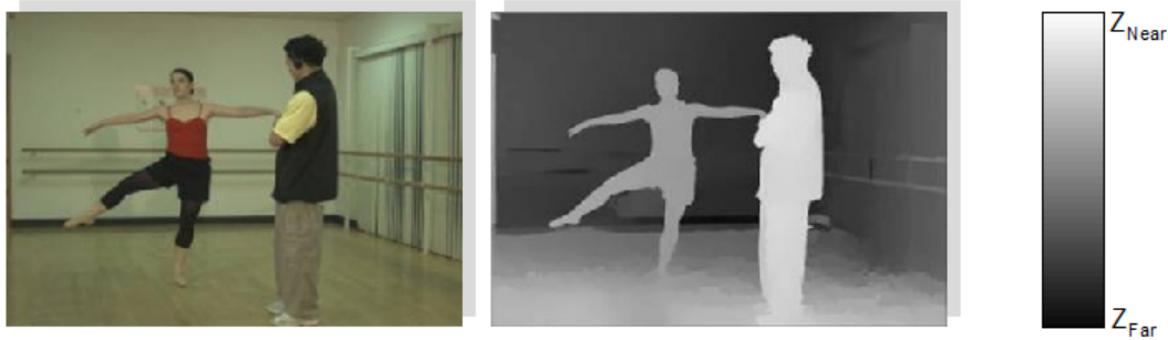
Figure 2.3: Multiview Video plus Depth representation consisting of a set of 2D color video views and their associated depth data
