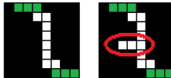
Figure 4.8: Example of a correct path (left) and an incorrect path with a branch (right). In both cases Ini and End sets are marked with green
