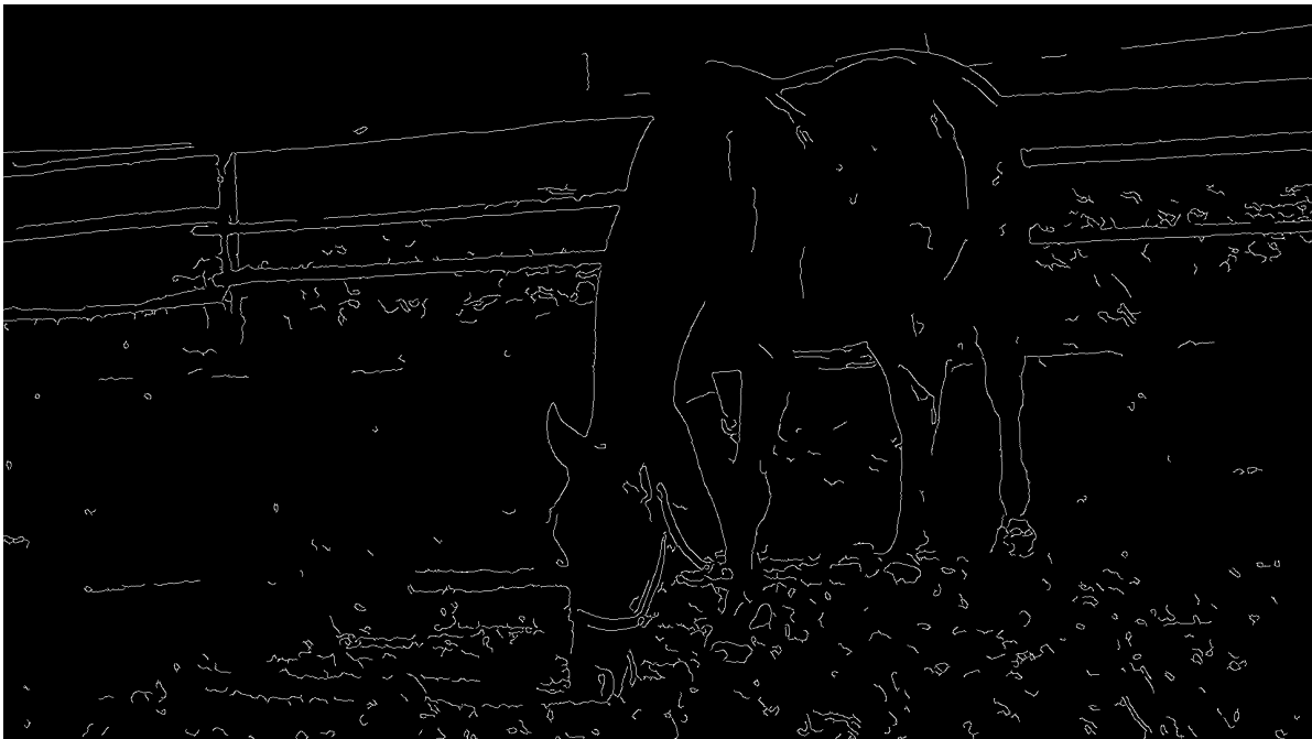
Figure 4.5: Canny output for Horse sequence. Grass (rough texture) is detected as edge information.
