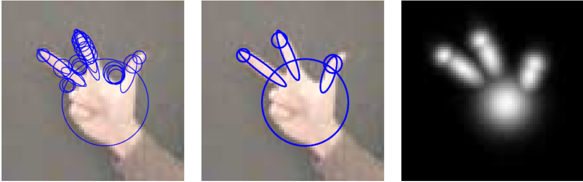
Figure 5.7: Image by Bretzner et al. (2002). They used multi-scale analysis to compute blob and ridge features to characterize the hand's geometry.
