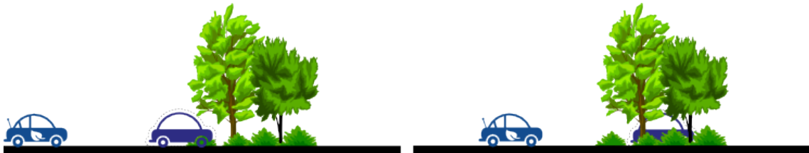
Figure 4.1: Location of two cars at a time step t (left) and at t + 1 (right). Suppose we are following the car on the right. Segmentation only would detect that a car has disappeared while a motion estimator would be able to shortly follow the car even though it is occluded.
