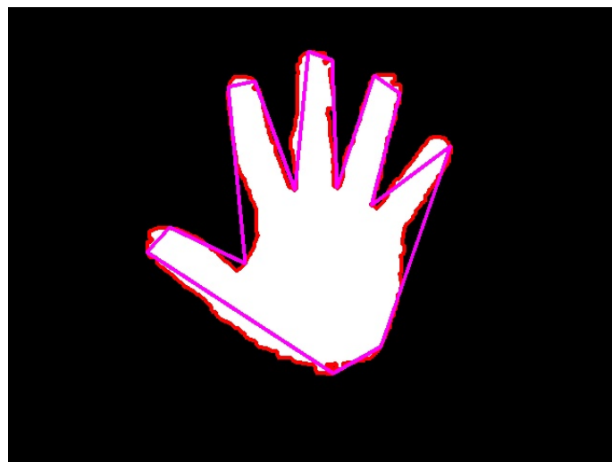
Figure 5.11: Polygonal approximation (purple lines) of the previous detected contour.
