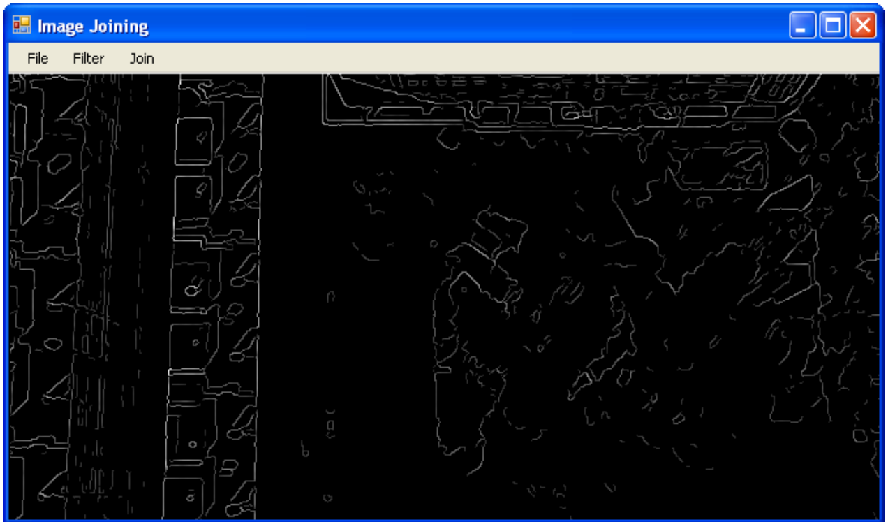
Figure 3.2.3: Image with Canny edge filter applied
