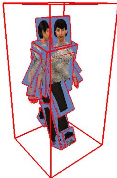
Figure 3.4: Collection of textures projected into the OBB faces.
