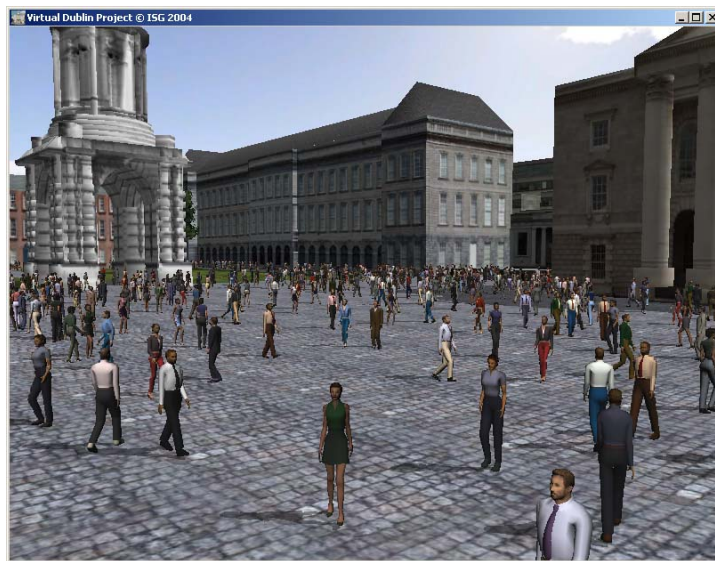
Figure 1.1: An example of a crowd simulation rendered with animated characters. Here distant agents are rendered by precomputed impostors. [12]
