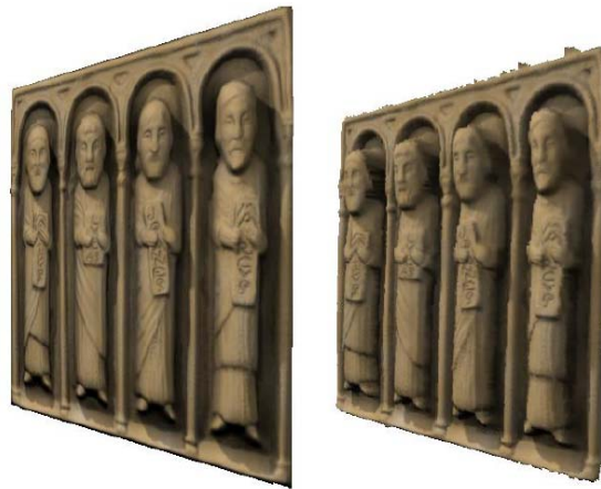
Figure 2.13: Color image rendered as a conventional texture (left) and relief texture mapped on one polygon (right). [25]
