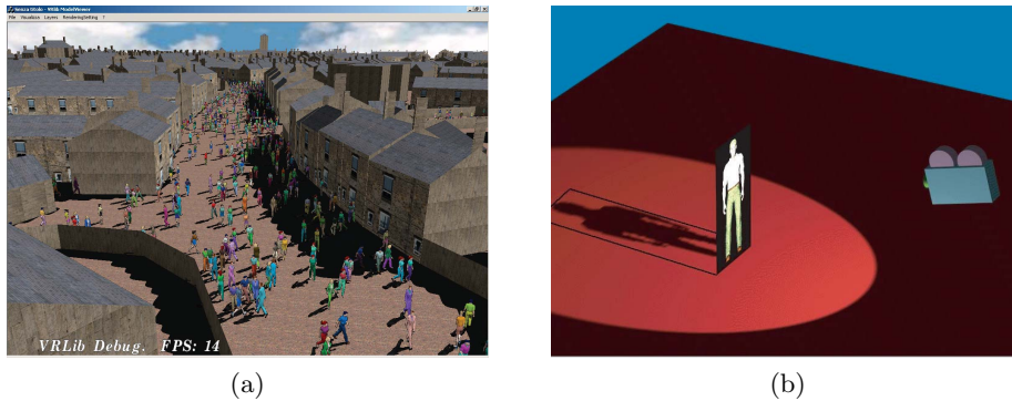
Figure 2.5: A scene with shadowing pre-generated impostors (a). The shadow of each agent is the projection onto the ground of the character's silhouette (b). [31]
