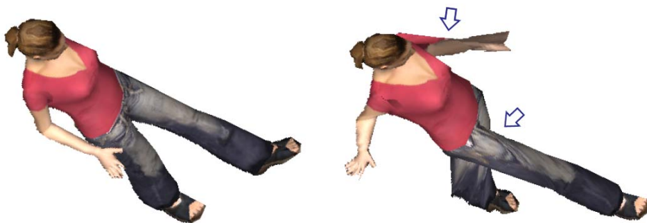
Figure 2.10: The Polypostor texture is generated from the first key-frame (left) and deformed for subsequent key-frames, producing artifacts due to lack of data in areas that have become visible (right). [17]
