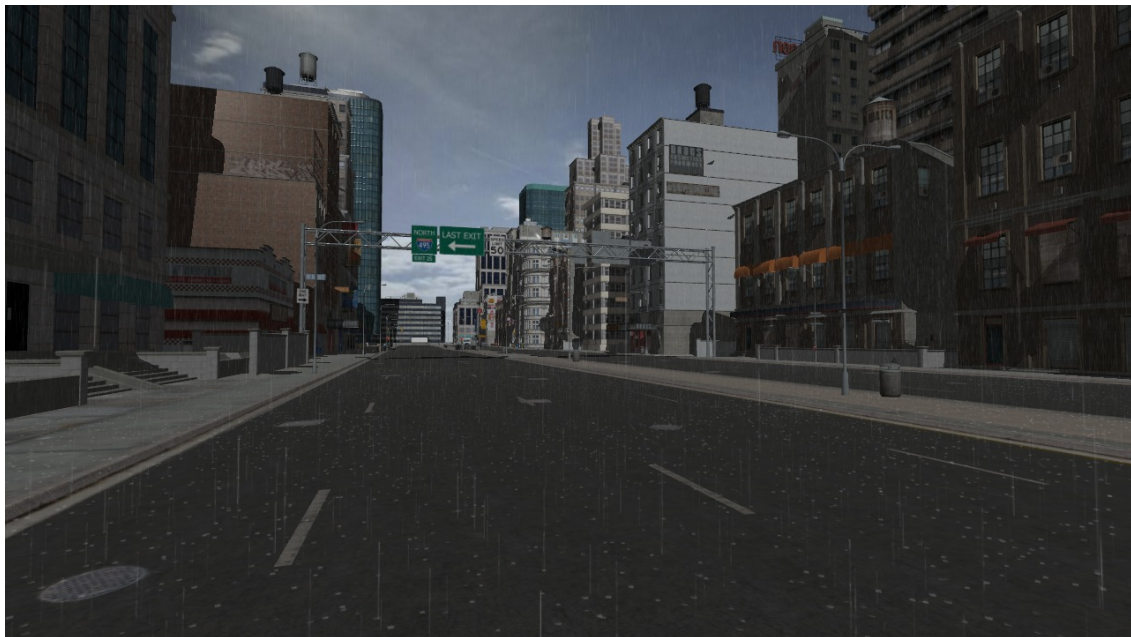
Figure 5.4: Renders obtained during the culling radius tests of Subsection 5.2.2 . The first image uses a radius of 5 meters; notice that rain disappearing in the vicinity can be perceived (specially by looking at the splashes on the ground). Second image uses a 20 meter radius and this artifact is no longer visible.
