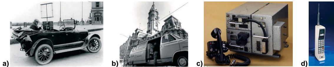
Figure A.2: a) 1924. Bell Labs tested mobile radio telephony, b) Early 1970s-Bell System tested the cellular concept, which had already been used in a commercial system since 1969, c) 1956. Original mobile phone from SRA (Svenska Radioaktiebolaget), d) The Motorola Dyna-TAC from 1983 was the first handheld cellular phone
