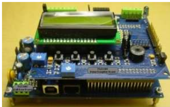
Figura 4.2.2. Montaje placa Flex Full Board y placa Flex Demo Daughter Board
