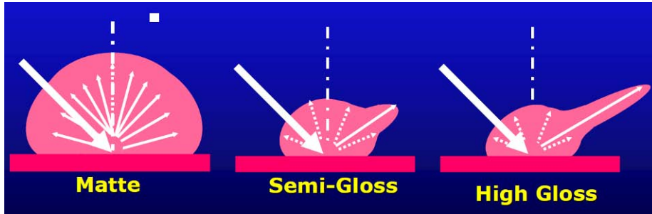
Figure 4-10 Gloss profiles for matte, semi-gloss and high gloss
