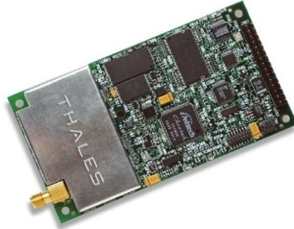
Figura 3.17 Receptor GPS DG14 Board de Magellan
