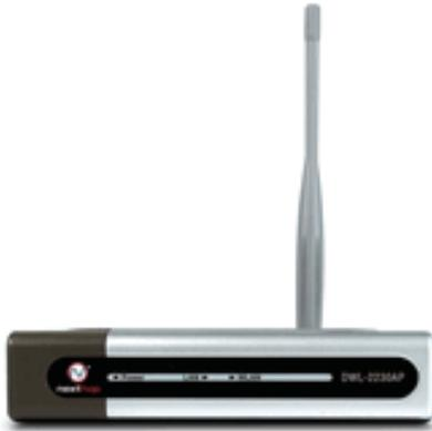
D-Link DWL-2230AP Access Point is designed specifically for business-class environments such as large or enterprise corporations, to provide secure and manageable wireless LAN options for network administrators.
