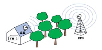
The Base Station represents the gateway allowing all the users connection to the WiMAX network: it provides coverage to all the Subscriber Stations in their area of influence and manages the traffic to and from these. The Terminal Equipment (e.g., a personal computer) is connected to the Subscriber Station to deliver it via packet traffic to the Base Station that will care to send it to the final recipient.
