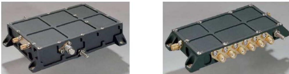
Fig. 3.13 Noise source (left) and power divider (right) (Credits: ESA).
