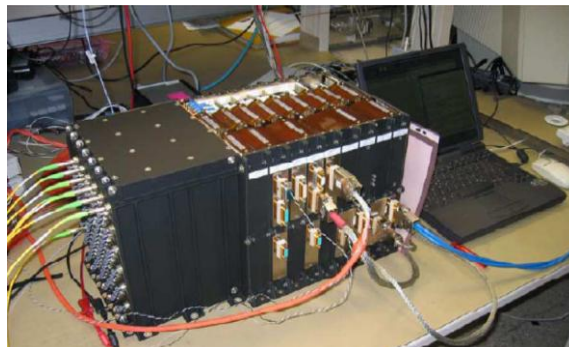
Fig. 3.15 Photograph of Correlator Control Unit (Credits: ESA).
