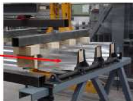
Figure 22: Local failure at the supports.
