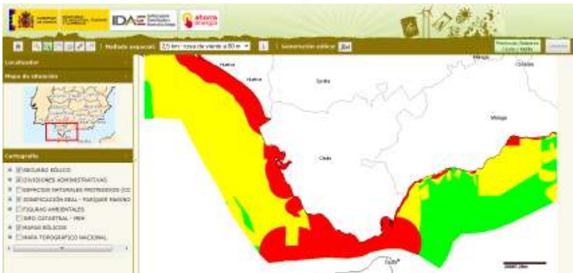
Figure A.2.1 Map of the zoning of offshore areas. In red exclusion zones, in yellow with restriction and in green suitable areas.
