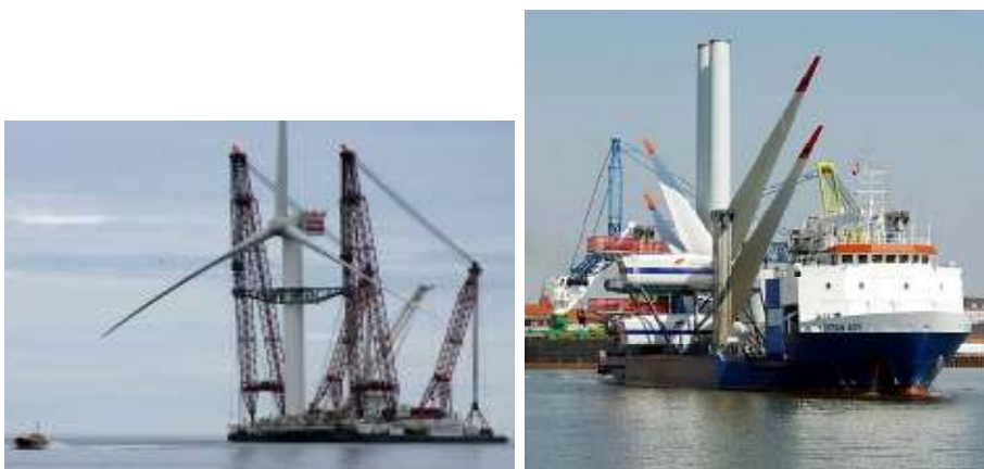
Figure 4.1.3 Transport of the turbine Horns Rev (left) and Beatrice (right).
