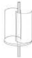
Figures 3.2.2 and 3.2.3 Sabonius (top and front view)
