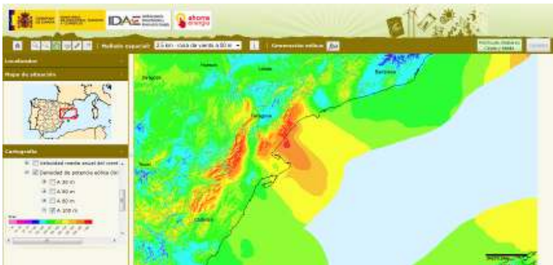
Figure A.3.7 Wind power density at 100m [W/m 2 ].
