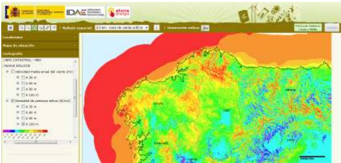
Figure A.1.7 Wind power density at 100m [W/m 2 ].
