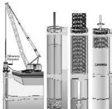
Figure 4.3.11 Construction of drilled shaft. From left to right, install casing and auger drill, place reinforcement cage, and pour concrete by tremie.
