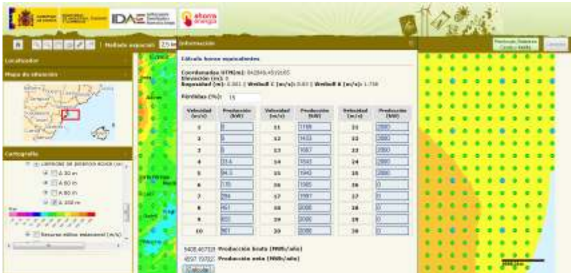
Figure A.1.17 Weibull parameters c and k with values of 8,83 and 1,736 m/s respectively. Gross annual production 5.408,47 GWh/year with V66-2MW wind turbine. Net annual production 4.597,19 GWh/year with V66-2MW wind turbine. [Calculated with IDAE's program]
