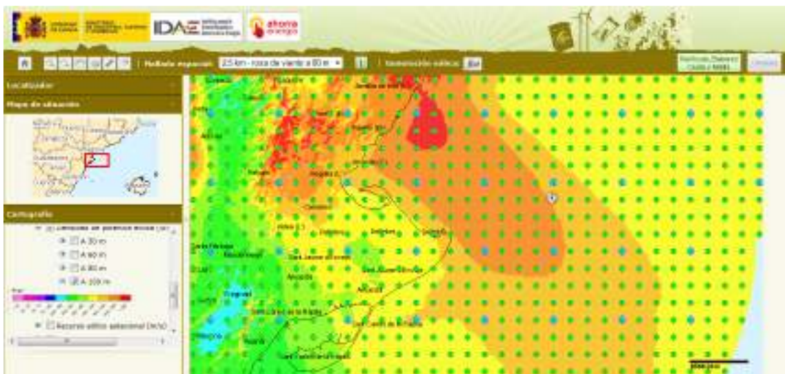
Figure A.3.15 Wind power density at 100m. In our study from 600 to 800 W/m 2 .
