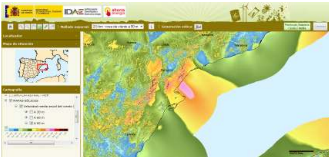
Figure A.3.2 Annual mean wind speed at 80 m [m/s].
