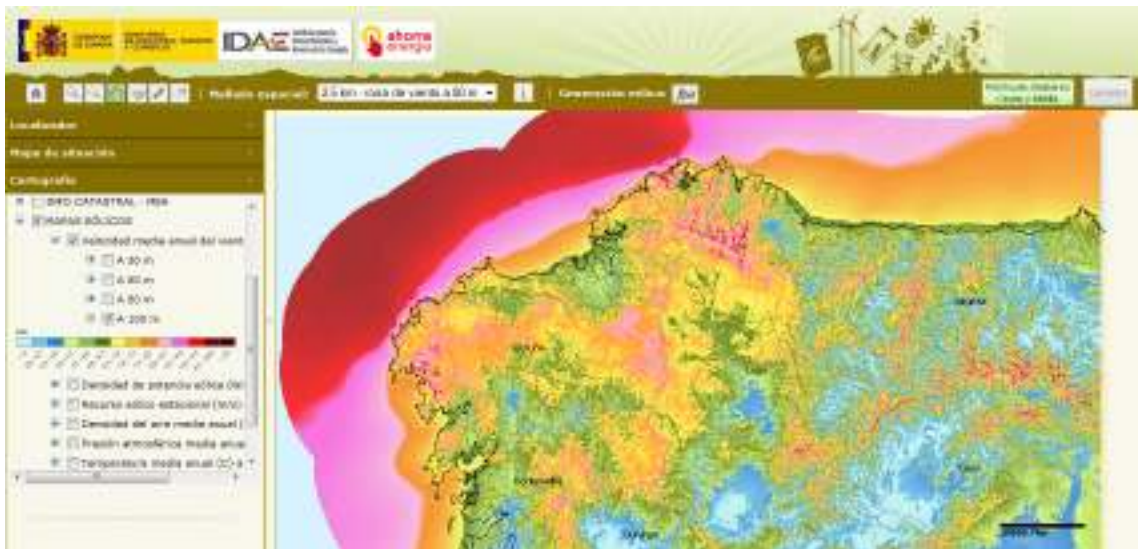
Figure A.1.3 Annual mean wind speed at 100 m [m/s].
