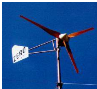
Figure 3.2.7 Wind vane method
