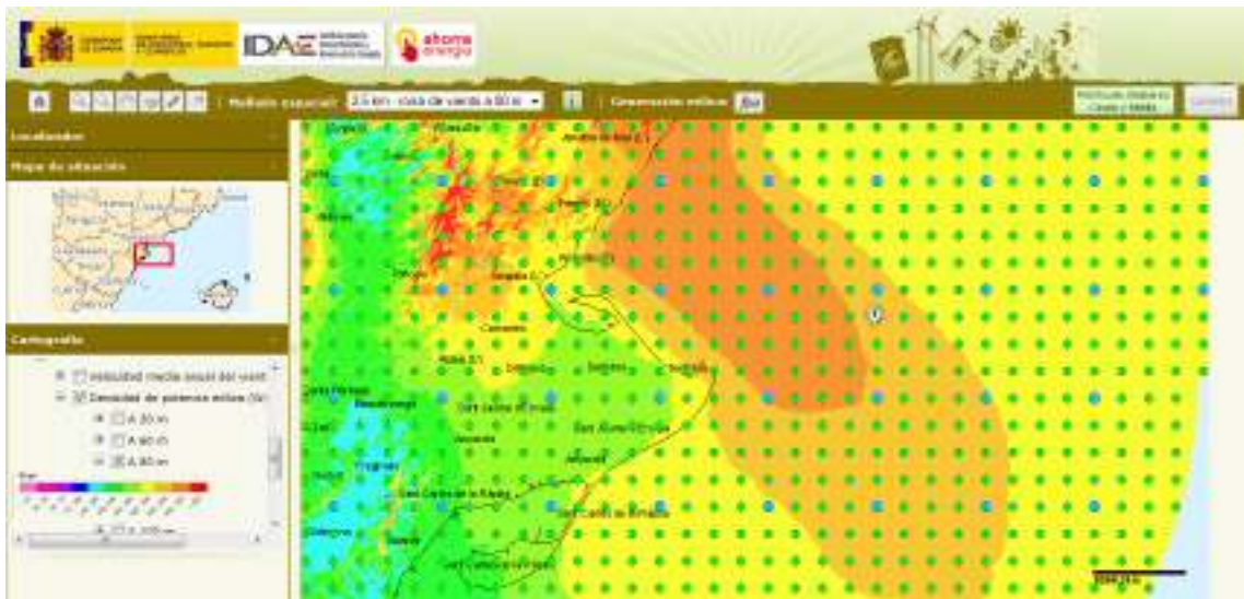
Figure A.3.14 Wind power density at 80m. In our study from 500 to 600 W/m 2 .
