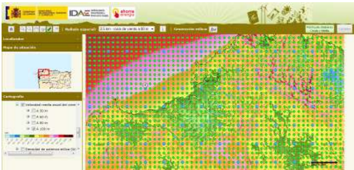
Figure A.1.14 Wind resource at 100m. In our study from 8 to 8,5 m/s.
