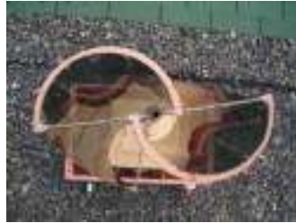
Figures 3.2.2 and 3.2.3 Sabonius (top and front view)
