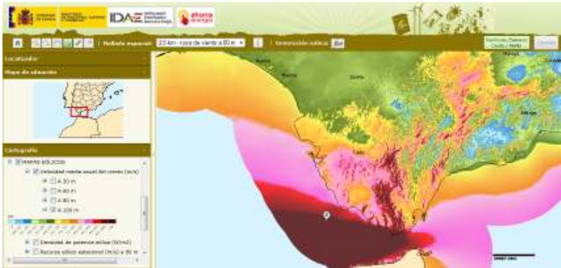
Figure A.2.13 Wind resource at 100m. In our study from 9,5 to 10 m/s.
