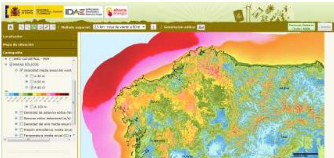
Figure A.1.2 Annual mean wind speed at 80 m [m/s].
