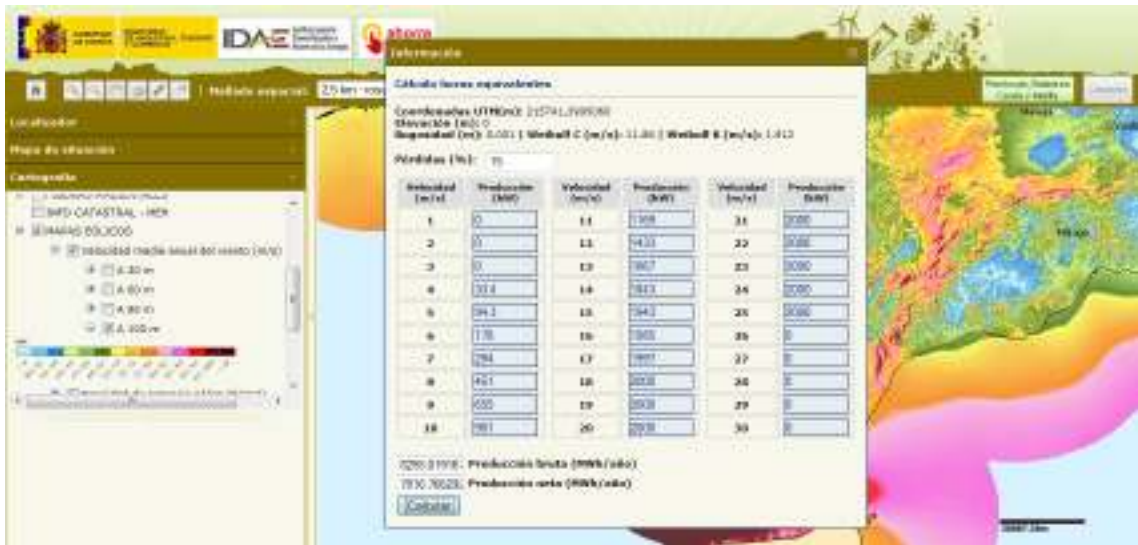
Figure A.2.16 Weibull parameters c and k with values of 11,86 and 1,912 m/s respectively. Gross annual production 8.255,01 GWh/year with V66-2MW wind turbine. Net annual production 7.016,76 GWh/year with V66-2MW wind turbine. [Calculated with IDAE's program]
