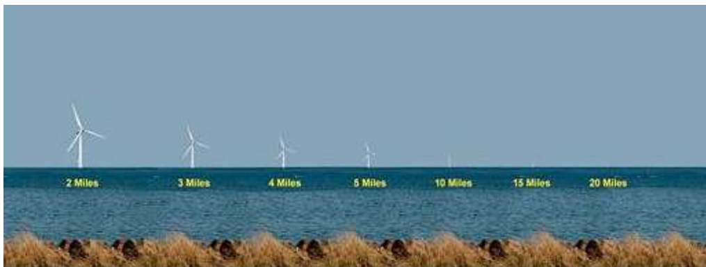
Figure 4.2.3 Graphic simulation of the wind turbine increasing the distance from the coast. It has to be taken into account that at a distance of 10 miles (16.09 km) the visual impact is very low. Weather must also be considered as the fog and mist could further reduce the visual impact.
