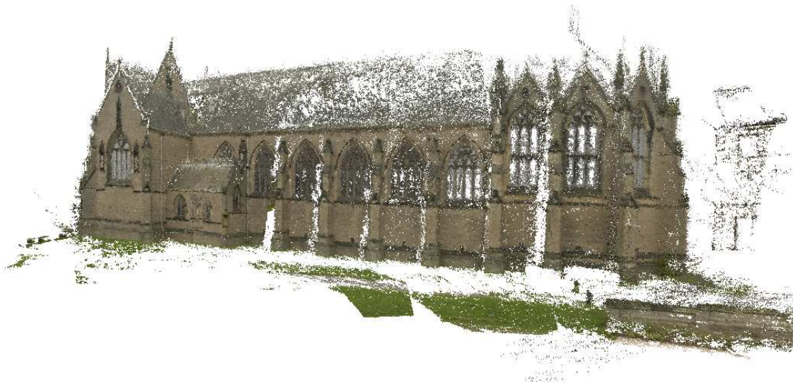
Figure 1: Model reconstructed from a set of photographs, notice that it is a point cloud model
