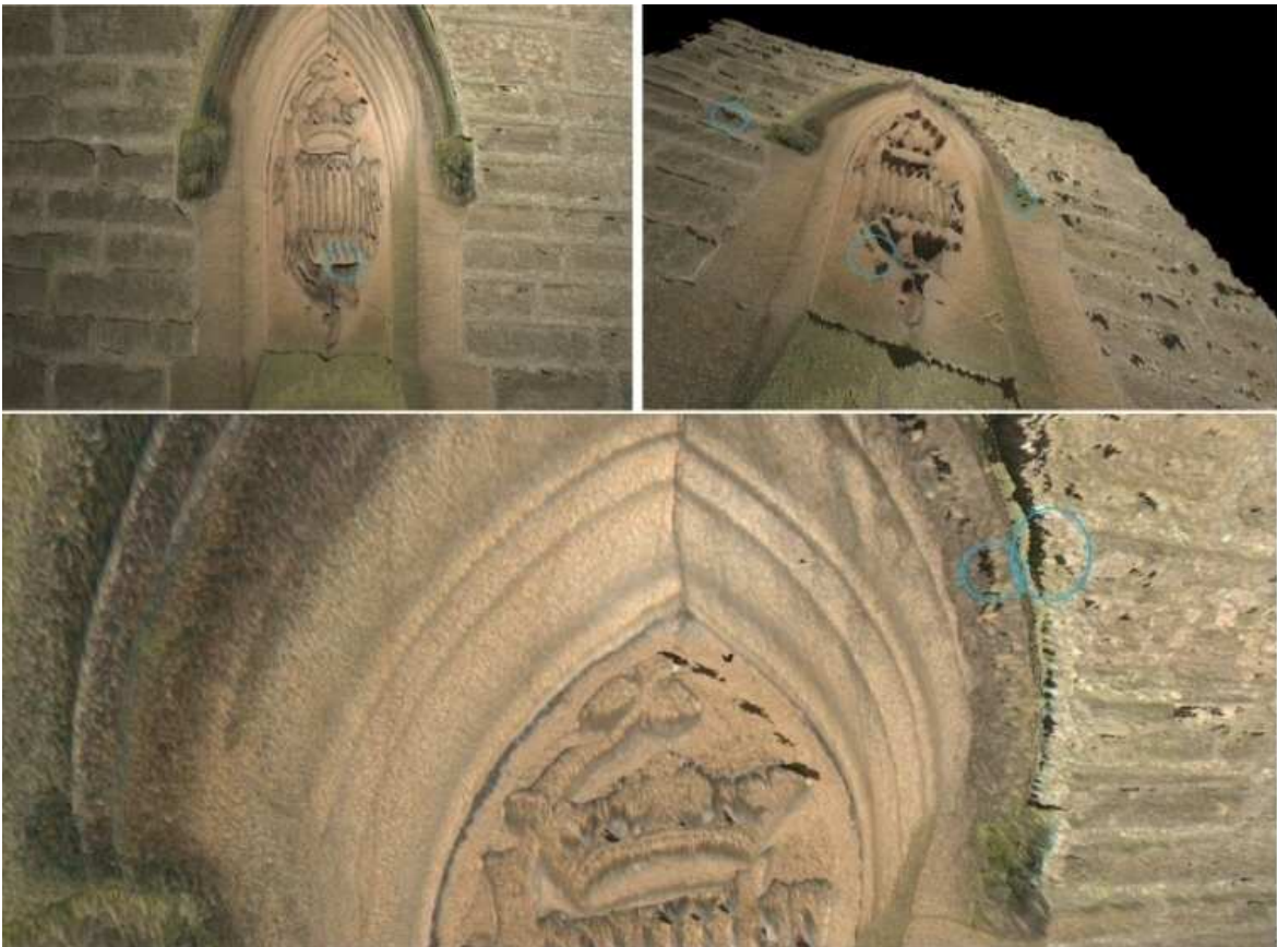
Figure 43: Visualization of a model using interval mapping. Notice the hard shadows when we look perpendicular (above left) and the artifacts in the shadows when we look from grazing angles (above right). Notice also how the shadows are not realistic at all (down) as they seem to be points instead of a continuous shadow due to the point light.
