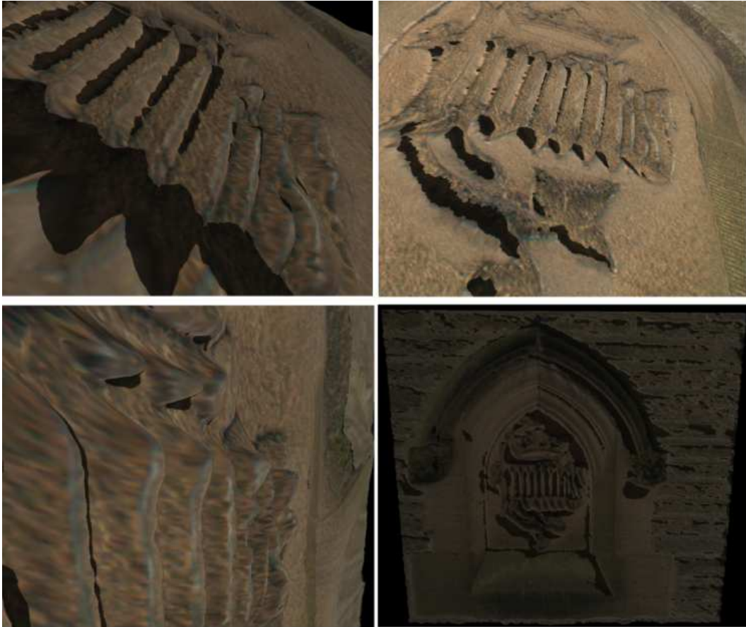
Figure 44: Images rendered using relaxed cone mapping, notice the hard shadows and the absence of artifacts even at grazing illumination or viewing angles
