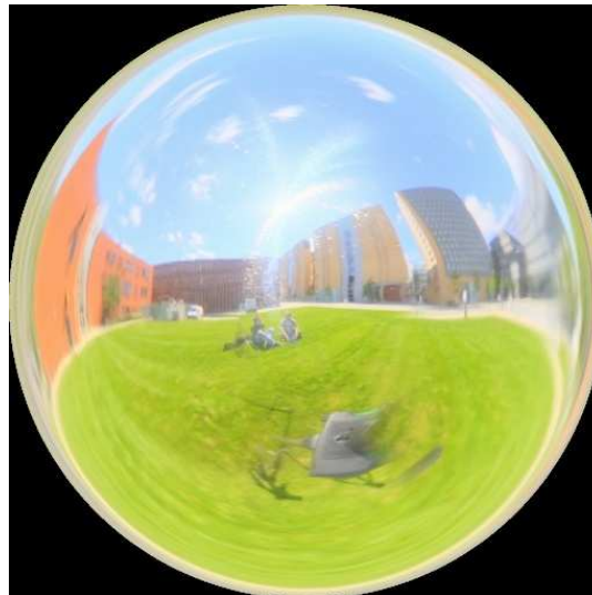
Figure 53: Light probe after the process. Notice that there is no camera and the regions of undersampling around the image have been improved
