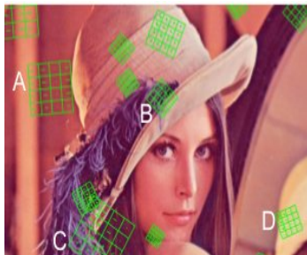
FIGURE 3.6: SIFT features on an image
