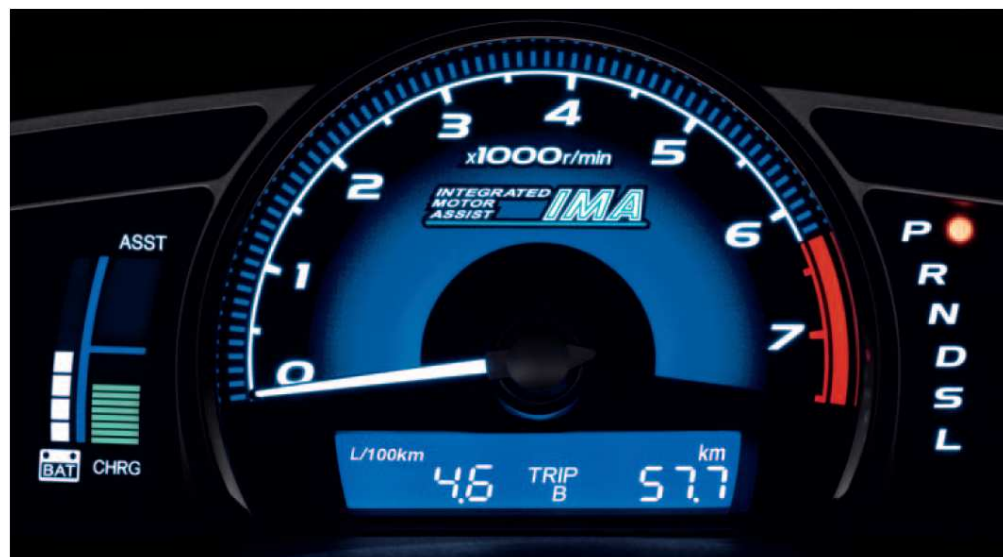
Fig. 4.4: Honda Civic Hybrid Dashboard Display.
