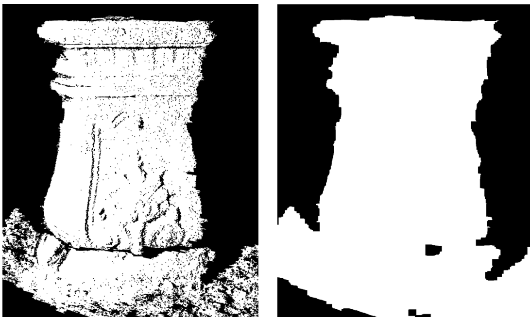
Figure 24: Left: Mask after blob filtering. Right: Resulting mask after erosion / dilation process.
