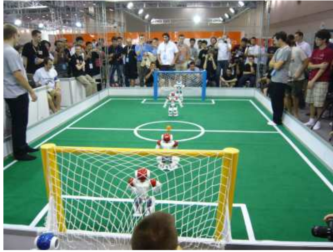
Figure 6.8: RoboCup game field where environment elements and game field have the same colours.
