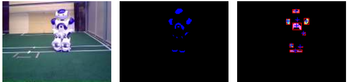
Figure 8.7: Nao detection process
