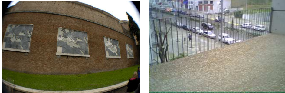
Figure 6.3: (a)Left: Image with fish-eye distortion that is easily observable in image corners. (b)Right: Image acquired with forehead Nao's camera.
