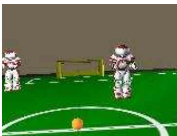
Figure 8.9: Nao image acquired with webots simulator (160x120 pixels)
