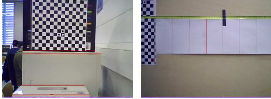
Figure 6.7: Two images from a set used for calculate horizontal FOV.
