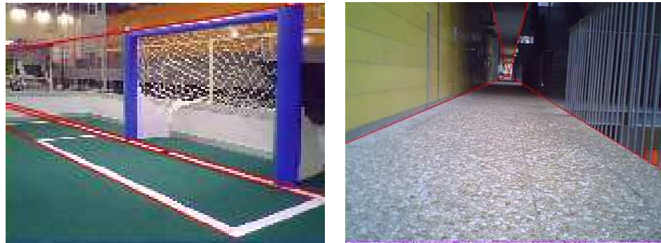
Figure 6.5: Images acquired with Nao robot. Images with principal rays on it crossing at vanishing point.
