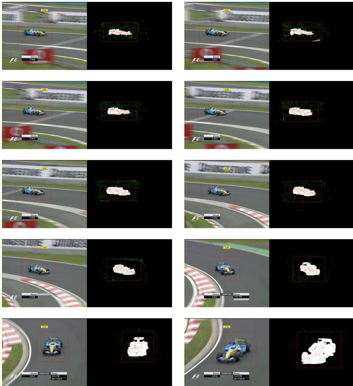
Figure 14 F1 car foreground segmentation 10 Gaussians model the foreground and 10 Gaussians model the background. This is a sequence with camera motion, object movement and scale change
