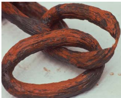
Figure 4 A corroded wrought iron chain. Figure 5 A corroded steel
