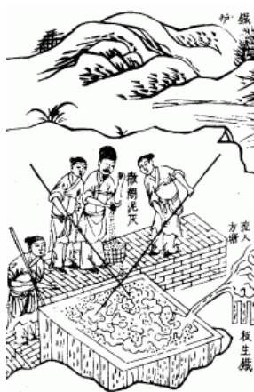
Figure 3 The puddling process of smelting iron ore to make wrought iron from pig iron. Tiangong Kaiwu encyclopedia published in 1637, written by Song Yingxing (1587-1666).
