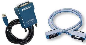
Fig. 3.9 GPIB cables to interconnect the PC to devices and the devices between them
